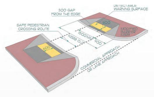
Figure 59: Kerb Cut Configuration Aligned
