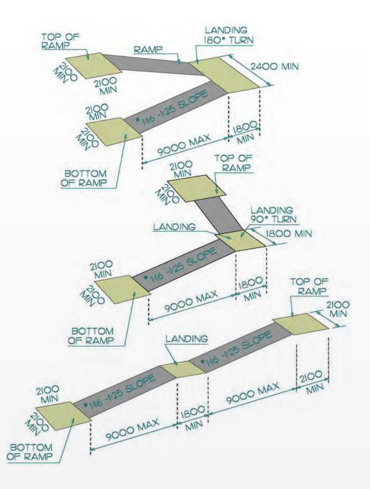
Figure 93: Minimum Ramp Landing Dimensions
