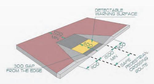
Figure 60: Kerb Cut Configuration Typical
