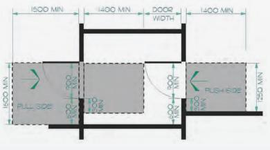
Figure 120: Manoeuvring Space at Doors in Series
