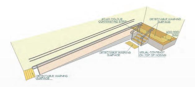
Figure 190: Detectable Warning Surfaces at Raised Platforms
