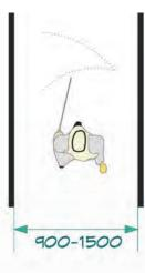
Figure 7: Clear Floor Space for a Person using a Long White Cane
