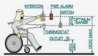
Figure 197: Reach Range for Accessible Controls
