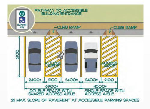
Figure 72: Perpendicular Parking Spaces
