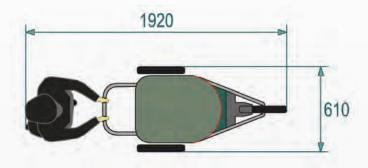
Figure 27: Clear Floor Space for a Single Jogger Stroller
