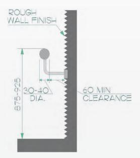
Figure 205: Handrail at Rough Wall
