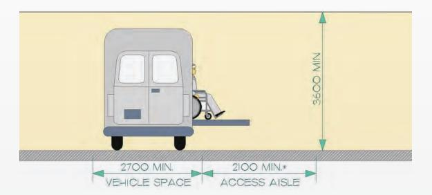
Figure 76: Height Clearance at Passenger Loading Zone
