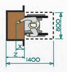
Figure 21: Forward Reach over an Obstruction
