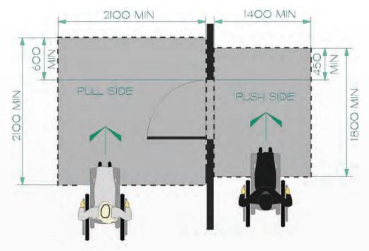
Figure 116: Hinge Side Approach at Hinged Doors
