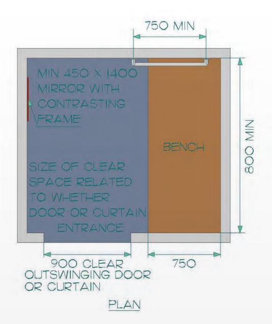
Figure 170: Floor Plan of Dressing Rooms
