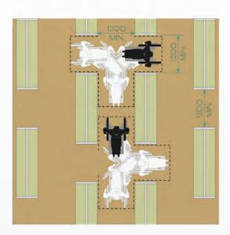
Figure 225: Aisle Width
