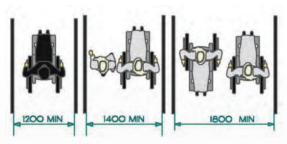
Figure 92: Access Widths
