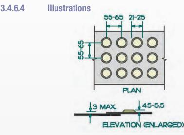
Figure 218: Truncated Dome Detectable Warning Surface
