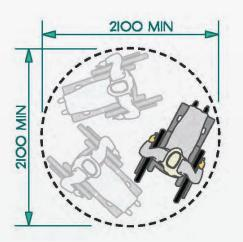
Figure 11: 360° Turning Space for Wheelchair
