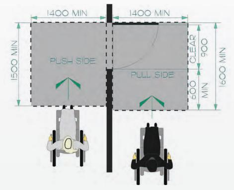
Figure 117: Latch Side Approach at Hinged Doors
