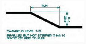
Figure 174: Changes in Level between 7 and 13 mm
