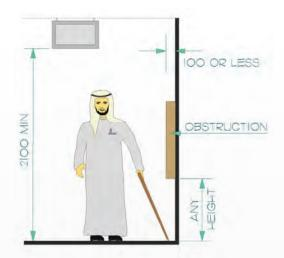
Figure 41: Limits of Protruding and Overhanging Objects
