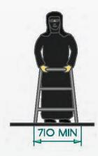
Figure 6: Clear Floor Space for a Person using a Walker
