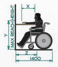
Figure 22: Forward Reach over an Obstruction
