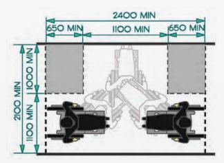
Figure 12: 3-Point Turning Space for Wheelchair or Mobility Scooter
