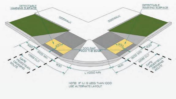
Figure 58: Kerb Cut Configuration at Corner
