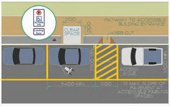
Figure 78: On-Street Passenger Loading Zone
