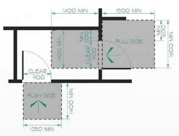
Figure 121: Manoeuvring Space at Doors in Series
