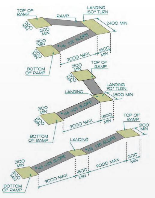
Figure 47: Minimum Ramp Landing Dimensions
