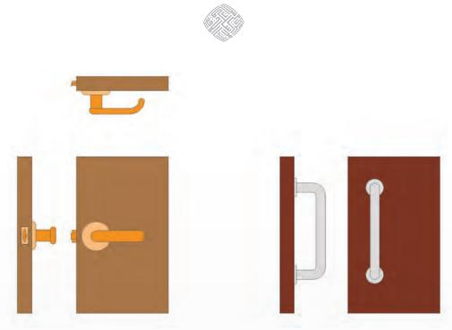
Figure 124: "U" shaped lever and "D" shaped handle.
