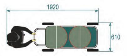
Figure 29: Clear Floor Space for a Twin Tandem Stroller
