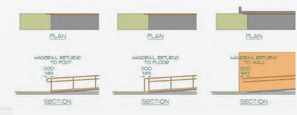
Figure 49: Horizontal Handrail Extensions
