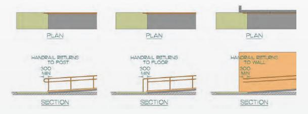
Figure 95: Horizontal Handrail Extensions
