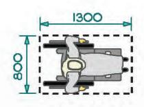
Figure 8: Clear Floor Space for a Person using a Manual Wheelchair
