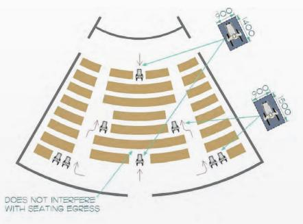
Figure 189: Distribution of Accessible Viewing Spaces
