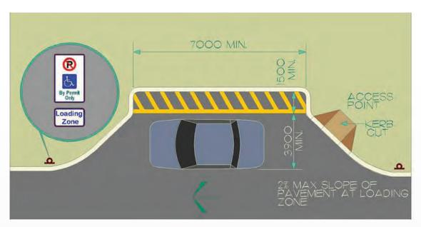
Figure 77: Off-Street Passenger Loading Zone
