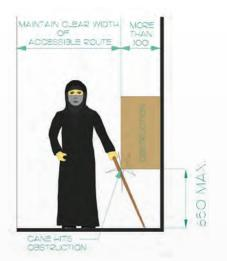
Figure 40: Limits of Protruding Objects
