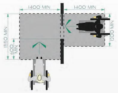
Figure 119: Front and Side Approach at Sliding Doors
