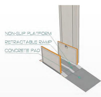
Figure 109: Vertical Platform Lift
