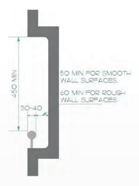
Figure 206: Handrail in Recess
