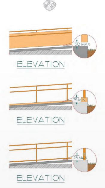
Figure 50: Edge Protection at Ramps
