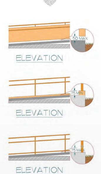
Figure 96: Edge Protection at Ramps
