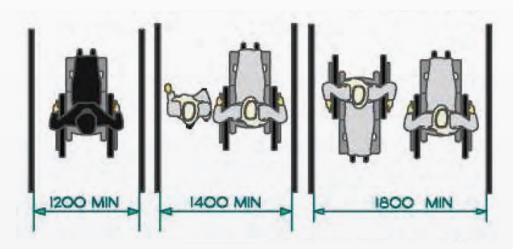
Figure 46: Access Widths
