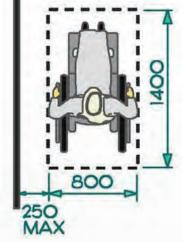
Figure 19: Side Reach - Maximum Distance to Wheelchair
