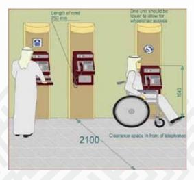
Figure 45. Accessible Phone Bank with One Lowermounted Public Phone to Accommodate a Person in a Wheelchair/Scooter
