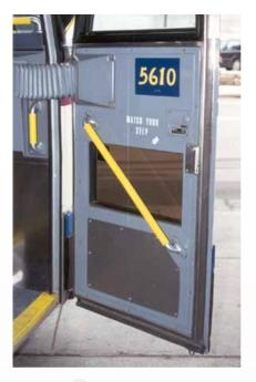
Figure 124. Colored Step Edge and Handrail
