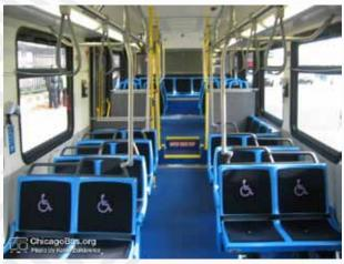
Figure 6. Partial Low Floor Bus - Chicago, Illinois, USA Source: www.chicagobus.org
