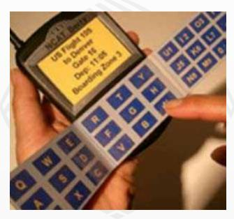
Figure 37. PDA Concept with Large Controls and Text Display Personal Digital Assistants (PDA) with large keys for persons with agility problems. Source: Rutenberg Design Inc., Canada
