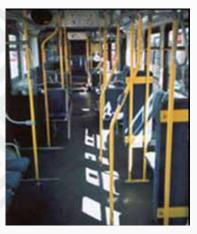
Figure 96. Colored Stanchions in Bus with High Color Contrast, OC Transpo, Ottawa, Canada - Source: Rutenberg Design Inc
