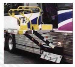
Figure 126. Storable Lift Mechanism
