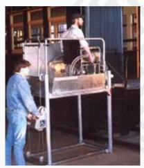
Figure 129. Station-Based Lift, VIA Rail in Ottawa, Canada Source: Rutenberg Design Inc.
