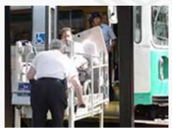
Figure 83. Station-based lift (used for boarding passenger in wheelchair from low platform to high vehicle floor, Baltimore, Maryland, USA)
