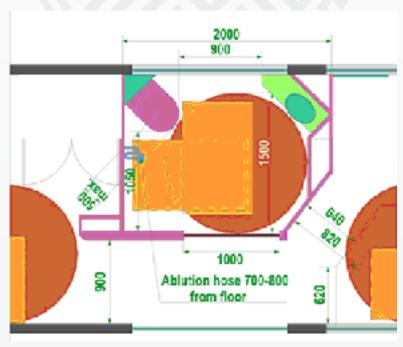
Figure 138. Accessible Washroom on intercity Rail Car
