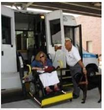
Figure-3. Accessible low floor community bus in Pennsylvania, USA.
