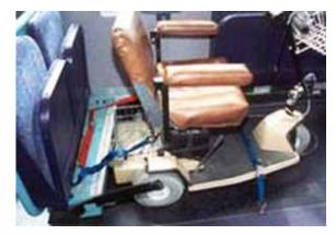
Figure 61. Wheelchair Securement Devices
