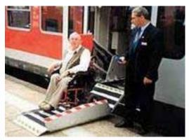
Figure 128. Onboard Operator-controlled onboard train lift in Sweden Source: www.railway-technology.com/contractors/passenger/u\_lift/
