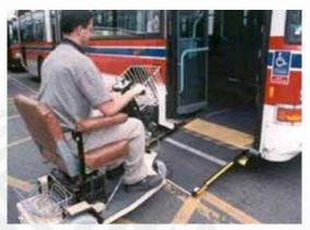
Figure 66. Scooter Access Over Ramp at Front Door to Kneeled Low Floor Bus from Road Level at BC Transit, Victoria, British Columbia, Canada
