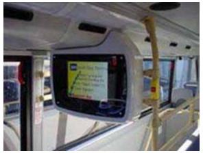
Figure 41. Onboard Destination Route Display on Intercity Bus Monitor, Canada
