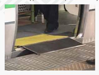
Figure 111. Bridge Plate in Rail Cars
