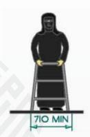
Figure 11. Clear Floor Space for a Person using a Walker
