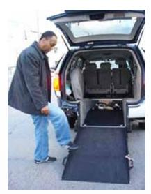
Figure 54. Ramp for Back Entry of accessible taxi in San Francisco, California, USA Source: UDA & Associates
