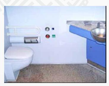
Figure 133. Accessible washroom on high speed ICE train in Germany
