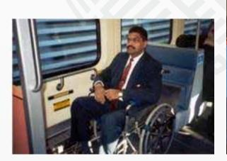
Figure 112. Wheelchair Space with Fold-Down Seat
