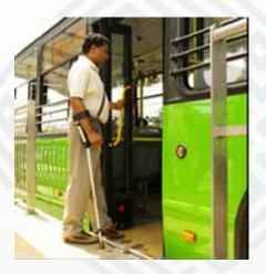
Figure 95. Vehicle to Platform Gaps. Person with Crutches Accessing BRT Vehicle in Delhi, India. (No bridge plate required) - Source: Samarthyam, India
