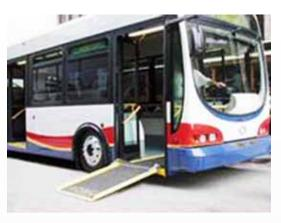
Figure 67. Attached Flip Ramp, Ricon Corp., USA/Canada
