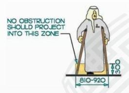
Figure 10. Clear Floor Space for a Person using Crutches
