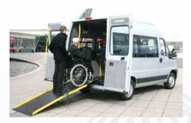
Figure-2. Minibus with ramp, rear access, Allied Mobility, UK. Source: www.alliedmobility.com
