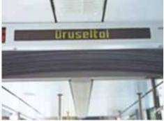
Figure 84. In-Vehicle information Text Display for Next Stop in LRT, Kassel Transit, Kassel, Germany
