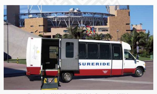
Figure 59. Special Vehicles Equipped With Lift or Ramp at Rear of Vehicle.
