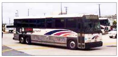
Figure 120. 14m Intercity coach with mid section access door, New Jersey Transit, USA
