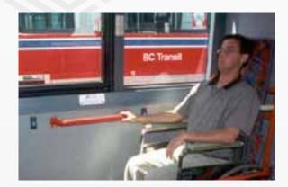
Figure 62. Handrail for Persons with Functional Limitations in a wheelchair position, BC Transit, Victoria, Canada Source: Rutenberg Design Inc., Canada
