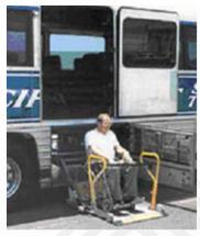
Figure 125. Vehicle-Attached Level Change Mechanism
