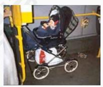
Figure 71. Wheelchair Position Used for Stroller When Not Occupied by a Wheelchair at Berlin Transit, Berlin, Germany
