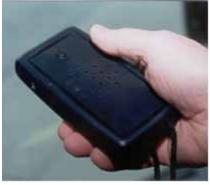
Figure 121. Infrared Transmitter at bus door and hand-held receiver for deaf/hard of hearing passenger to access information for bus number and destination.
