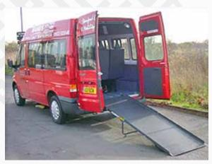
Figure 60. Foldable ramp at rear of minibus, UK Source: www.portaramp.co.uk
