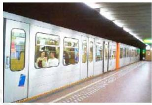
Figure 97. Metro Station in Brussels with Tactile warning strip on platform and color warning on cars.
