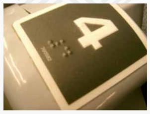
Figure 131. Train Seat Identification for Blind Persons, with raised number and in Braille on armrest, VIA Rail, Canada Source: Rutenberg Design Inc
