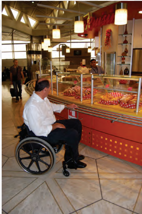
Figure 121: Lowered buffet and tray counters are important for accessibility Source: UDA & Associates
