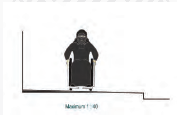
Figure 132: Minimum camber setup/ layout Source: UDA & Associates
