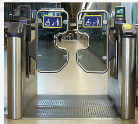
Figure 179: Access Gate Designed to Accommodate Mobility Aid
