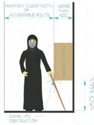
Figure 58: Limits of Protruding Objects
