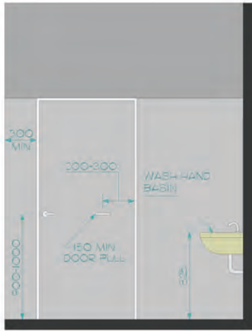
Figure 102: Accessible Toilet Stall
