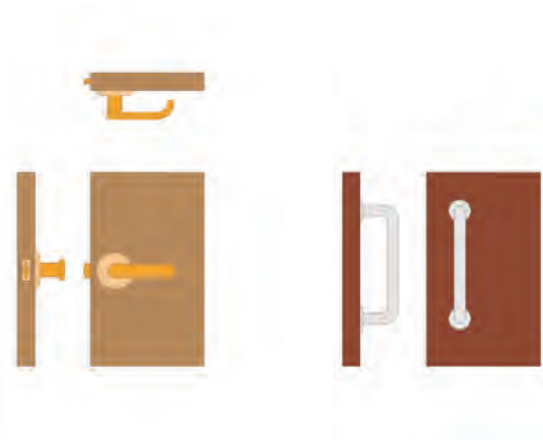
Figure 82: "U" shaped lever and "D" shaped handle. Source: UDA & Associates
