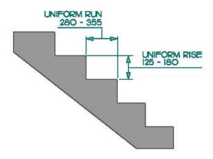
Figure 12. Riser Criteria (Unless otherwise noted, all dimensions are given in millimeters).
