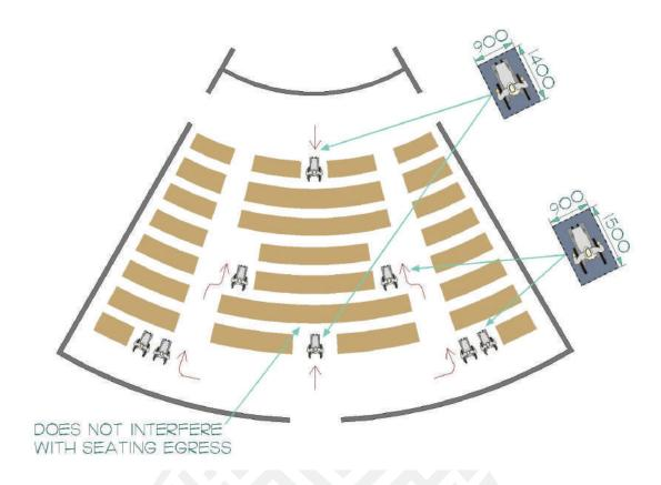
Figure 104. Distribution of Accessible Viewing Spaces. Dimensions in Millimeters.
