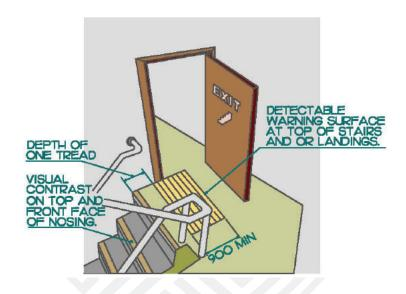
Figure 36. Detectable Warning Surfaces at Stairs. Dimensions in Millimeters.
