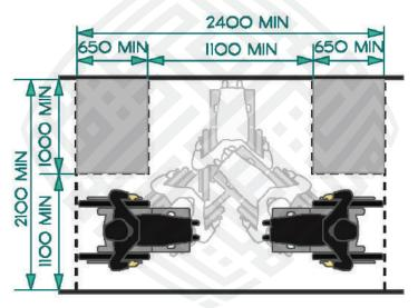
Figure 117. 180° Turning Space for Wheelchair or Scooter
