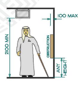
Figure 134. Limits of Protruding Objects
