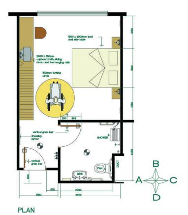
Figure 52. Typical Room Configuration.
