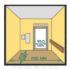
Figure 14. Elevator Cab (Unless otherwise noted, all dimensions are given in millimeters).
