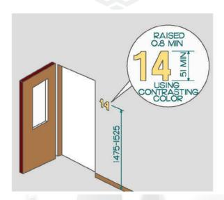
Figure 42. Tactile Lettering. Dimensions in Millimeters.
