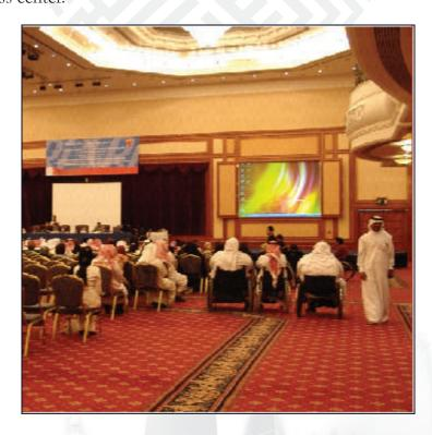
Figure 60. Example of accessible conferencing facilities, ideally the wheelchair seating should be integrated into the seating layout and not just provided on the sides
