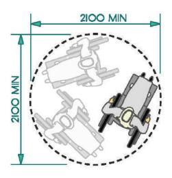
Figure 116. 360° Turning Space for Wheelchair or Scooter
