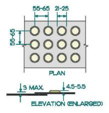
Figure 37. Truncated Dome Detectable Warning Surface. Dimensions in Millimeters.
