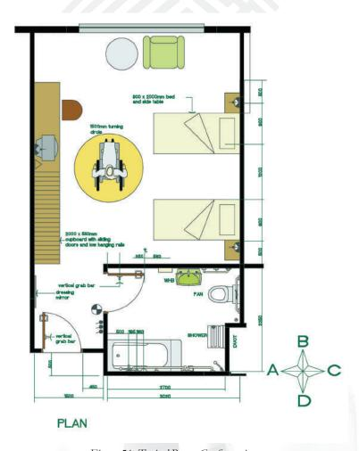
Figure 51. Typical Room Configuration.
