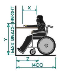
Figure 125. Forward Reach over an Obstruction
