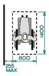
Figure 126. Side Reach - Maximum Distance to Wheelchair
