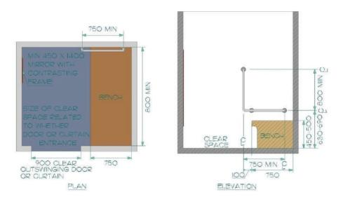
Figure 97: Private accessible dressing room. Dimensions in millimeters.
