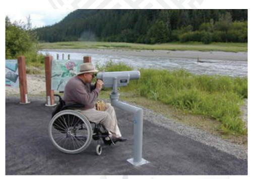
Figure 87. An example of a lowered telescope in use.
