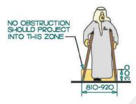
Figure 110. Clear Floor Space for a Person using Crutches
