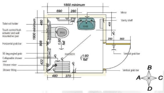
Figure 56. Typical Washroom Configuration.
