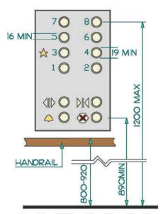
Figure 16. Control Panel (Unless otherwise noted, all dimensions are given in millimeters).
