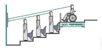
Figure 103. Sight-Lines at Wheelchair Locations. Dimensions in Millimeters.
