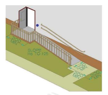
Figure 11. Ramp Criteria. Dimensions in millimeters.
