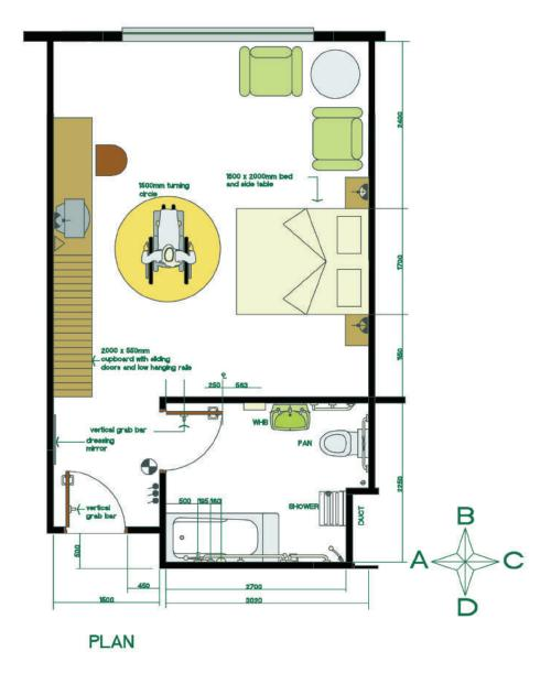
Figure 54. Typical Room Configuration.
