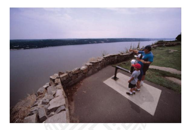
Figure 85. Designation of overlook areas and the provision of 'safe' areas with color-contrasting provides not only areas of use for seated users, but the achieved color-contrasting provides some level of warning of the position of telescopes and similar devices. The lowering of telescopes, as shown here, also allows children and seated persons to make use of such equipment.
