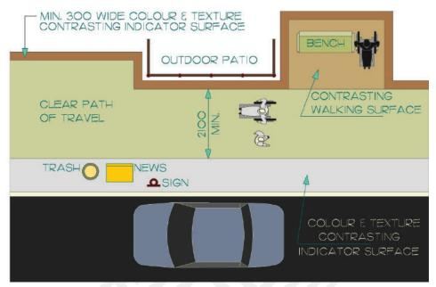
Figure 27: Streetscape. Dimensions in Millimeters.
