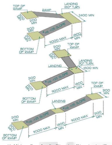
Figure 10. Minimum Ramp Landing Dimensions. Dimensions in millimeters.
