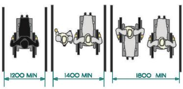
Figure 140: Access Widths
