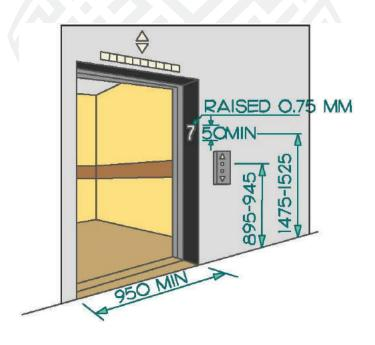
Figure 15. Elevator Entry (Unless otherwise noted, all dimensions are given in millimeters).
