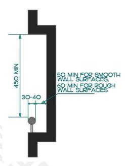
Figure 143. Handrail in Recess
