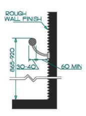
Figure 142. Handrail at Rough Wall
