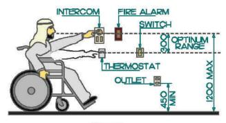
Figure 144. Reach Range for Accessible Controls
