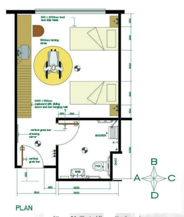
Figure 53. Typical Room Configuration.
