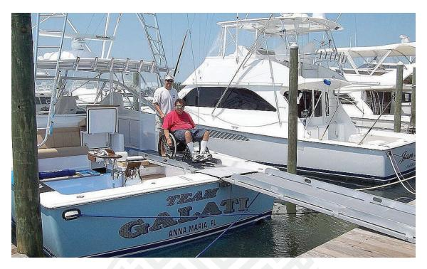
Figure 93. An example of specialized telescopic ramp providing access for a wheeled-user. Where environmental constraints are in place, the usage of specialized equipment is necessary; this underscores the need for the design of such facilities to incorporate principles of universal access from their initiation.
