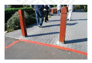
Figure 89. Using color to demarcate spaces, as well as differences in floor surfaces to indicate different usages, contribute to the usability of environments. This is also a good example of how bollards can be employed to stop vehicular traffic, yet still retain the sufficient width to allow assistive mobility devices to gain access.
