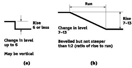
Figure 130. Changes in Level up to 6 Figure 131. Changes in Level between 7 and 13
