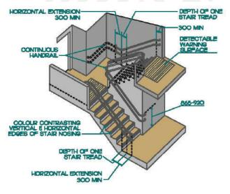
Figure 13. Stair Design Criteria (Unless otherwise noted, all dimensions are given in millimeters).
