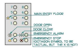
Figure 17. Tactile Symbols (Unless otherwise noted, all dimensions are given in millimeters).
