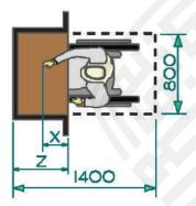
Figure 127. Forward Reach over an Obstruction
