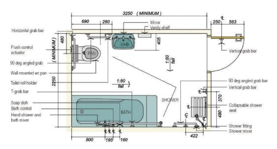
Figure 55. Typical Washroom Configuration.
